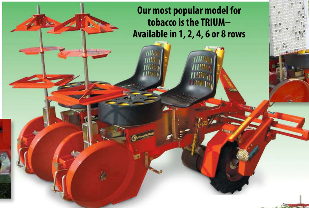
adjustable tension/parallelogram for constant planting depth
